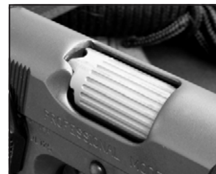
Ball-milled flutes function as sand cuts to work grit and sediment out from between the barrel and slide. A barrel hood port allows for a visual chamber inspection.
