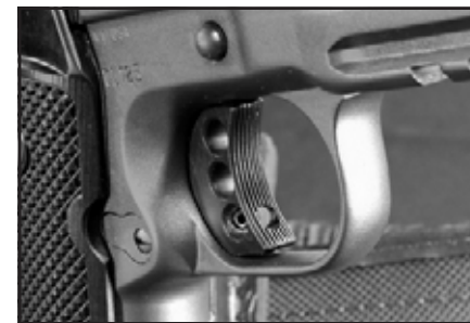
The adjustable trigger is D&L Sports' aluminum 3-hole unit with a serrated face.
