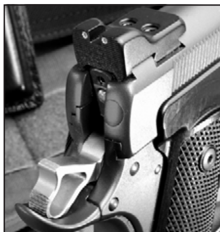
The rear sight is dovetailed into the slide, and set with dual screws. Note the dehorning and melting done to corners and edges.
