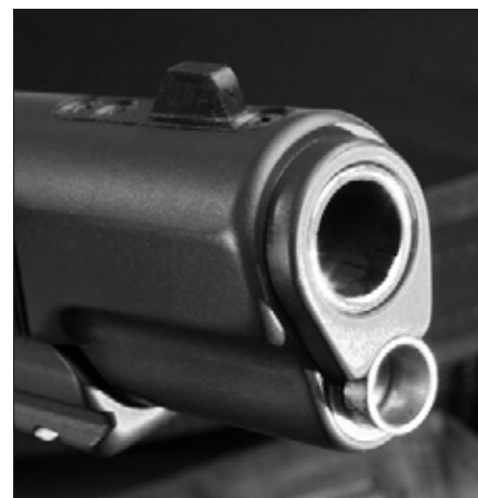
A D&L match barrel and bushing set are fitted for accuracy and functioning, and a bushing flange is used for durability.
